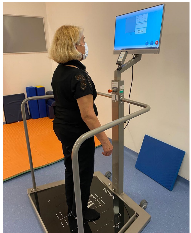
Figure 1. Patient positioning on the HUR SmartBalance device for static balance and proprioception testing.
